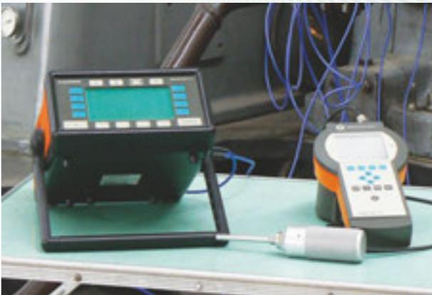
Periodical diagnostic measurements by means of a data collector to obtain a permanent survey of the vibration situation even in large machinery. Long-term data archiving on a PC, creating trends, monitoring changes of state after completed repairs, etc.
